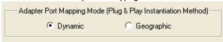
The **Adapter Port Mapping Mode** box allows you to change the behavior of how Keyspan COM port numbers are assigned when you connect the Keyspan adapter to a different USB port than the one it was originally connected to.
