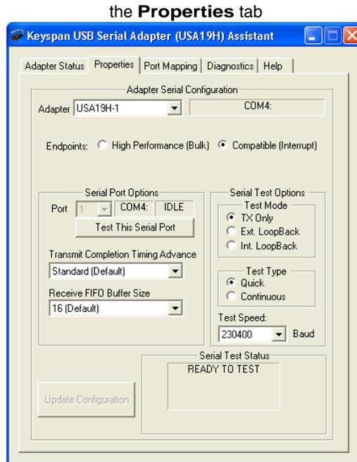
The **Properties** tab in the Keyspan Serial Assistant allows you **test** your Keyspan adapter and **make changes to the behavior** of the Keyspan adapter. The following is an explanation of the items in this tab.
