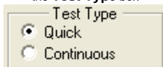
The **Test Type** box allows to specify how many times the selected test will be repeated when you press the Test button. Use the *Quick* option to perform the test once. To perform a subsequent test, press the **Test This Port** button. Use the *Continuous* option to repeat the test continuously. To stop the test, press the **Stop Test** button (the **Test This Port** button becomes the **Stop Test** button during a test).
