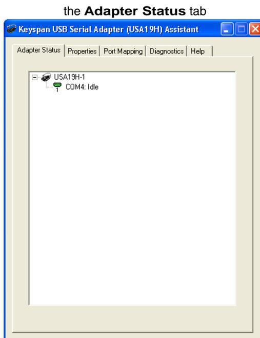
The **Adapter Status** tab in the Keyspan Serial Assistant displays the status of your Keyspan adapter. Specifically, it shows the *COM port number* (ie **COM1**, **COM2**, etc.) and the *COM Port Status*. (**IDLE** or **BUSY**). If you have several Keyspan adapters of the same type, they will all show up in this tab.
