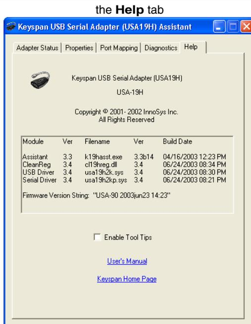
The **Help** tab in the Keyspan Serial Assistant displays the version numbers of the different components in your Keyspan USB Serial Adapter installation. You can also enable **Tool Tips** (on screen help), read your Keyspan adapter's User's Manual, or go to Keyspan's home page.
