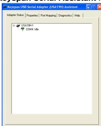
If your Keyspan hardware and software are installed correctly, you will see your adapter in the '**Adapter Status**' tab box. You should also see the *COM port number* (ie **COM1**, **COM2**, etc.) and the *COM Port Status*. (**IDLE** or **BUSY**).
