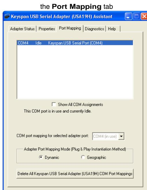
The **Port Mapping** tab in the Keyspan Serial Assistant allows you to change how COM port numbers are assigned to your Keyspan adapter. The following is an explanation of the items in this tab.
