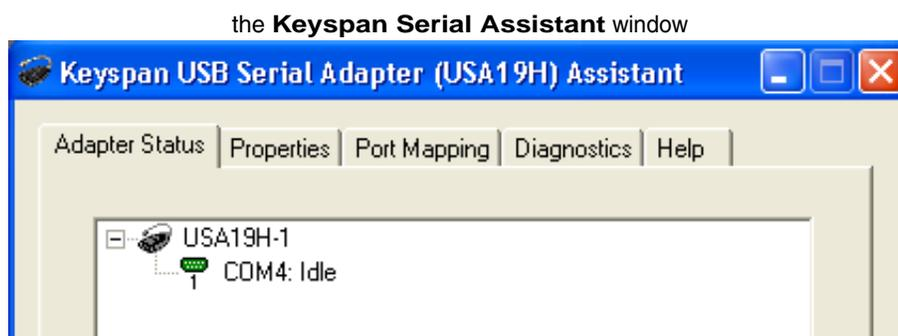
If your Keyspan hardware and software are installed correctly, you will see your adapter in the '**Adapter Status**' tab box. You should also see the *COM port number* (ie **COM1**, **COM2**, etc.) and the *COM Port Status*.(**IDLE** or **BUSY**).
