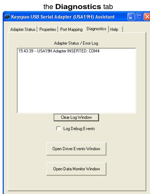
The **Diagnostic** tab in the Keyspan Serial Assistant reports diagnostic information about your Keyspan adapter's software and hardware. The following is an explanation of the items in this tab.
