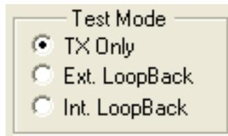
The **Test Mode** box allows to specify the type of test that will be performed when you press the **Test This Port** button.
