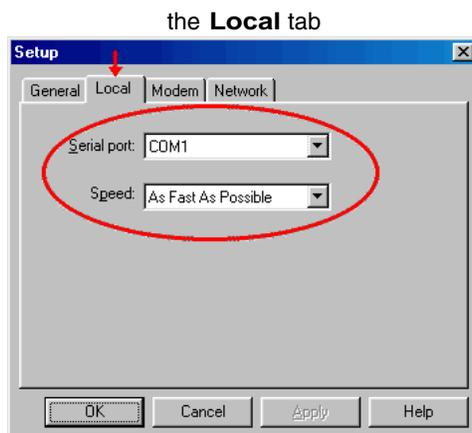
Select your Keyspan COM port in the **Serial port** pull down menu (see step 1 in this example).
