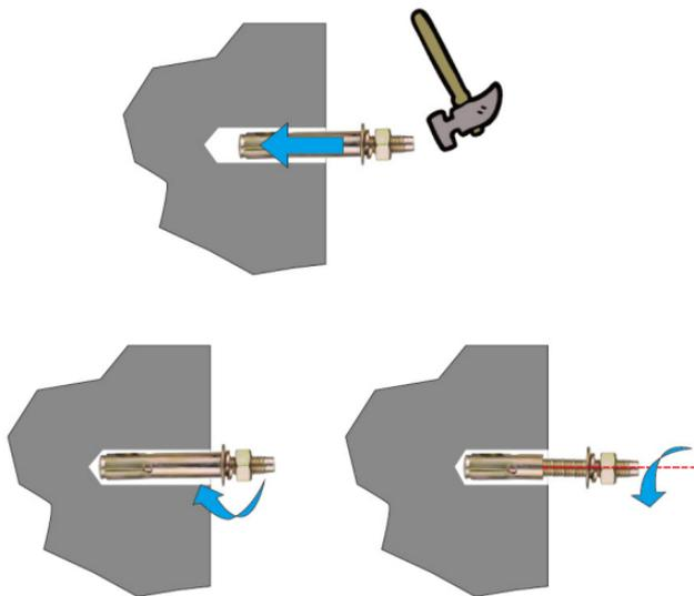
Figure 2-7: Install the expansion bolt
