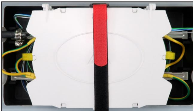
Figure 1-19: Close the splicing tray cover
