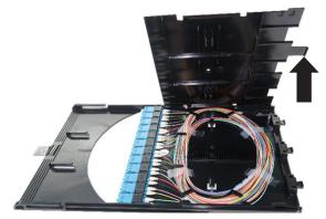
3. Splice the desired pigtail with the fiber drop cable in accordance with standard industry splicing practices.
