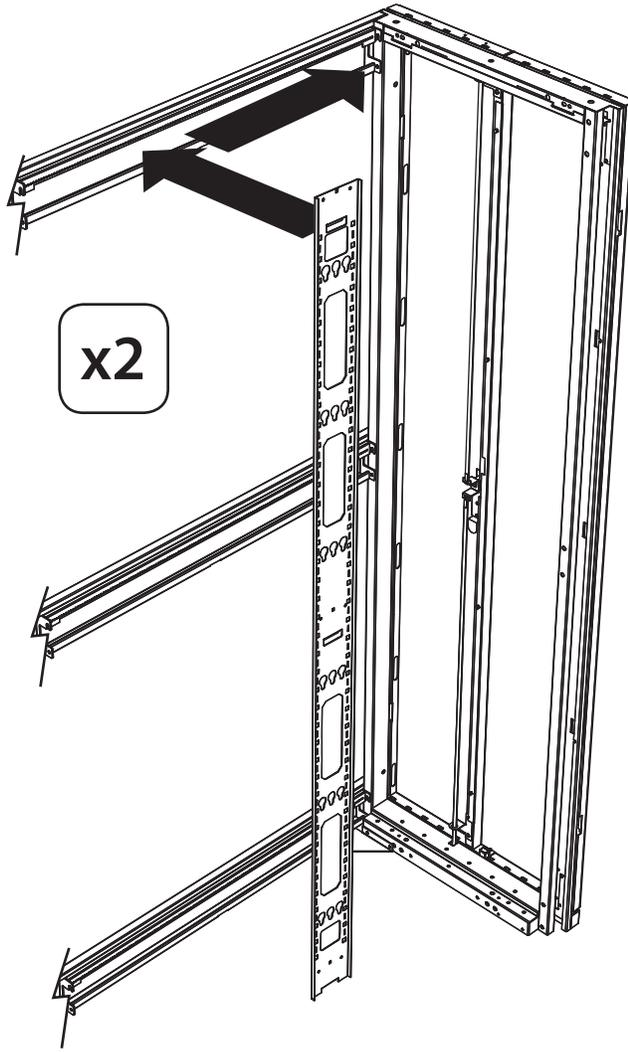
The rail attachment points are numbered to help you align each pair of rails at the same depth. Before attaching the rails using the screws (shown in Step 5-3), make sure the same number appears in all three windows. **Note: Number shown in Step 5-2 is for illustration purposes only; attach rails at desired depth.**
