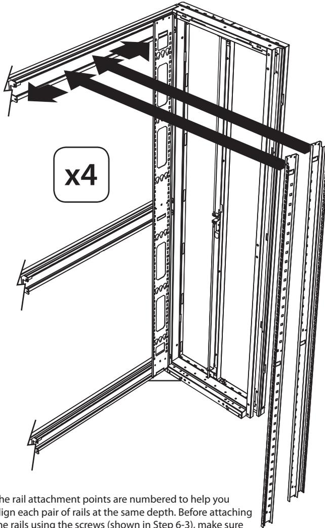
The rail attachment points are numbered to help you align each pair of rails at the same depth. Before attaching the rails using the screws (shown in Step 6-3), make sure the same number appears in all three windows. **Note:** Number shown in Step 6-2 is for illustration purposes only; attach rails at desired depth.
