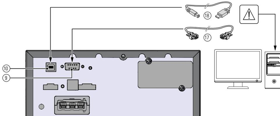
1. Connect the RS232 ⑰ or USB ⑱ communication cable to the serial or USB port on the computer equipment.
