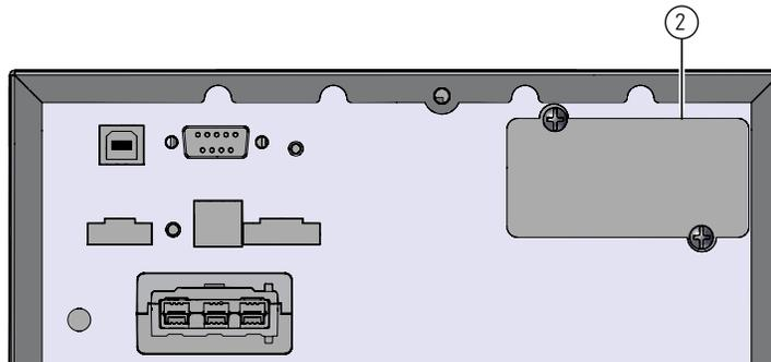
1. Remove the slot cover ② secured by screws.
