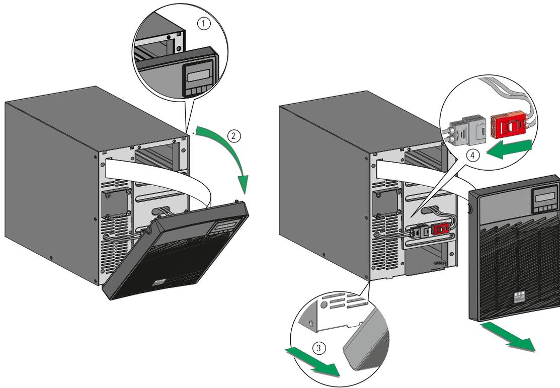
1. Unlock the holders on the upper part of the front panel.
