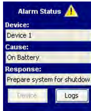
Figure 15: PowerAlert Local On Battery Alarm
