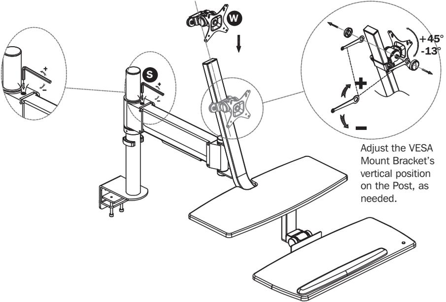
Adjust the VESA Mount Bracket's vertical position on the Post, as needed.
