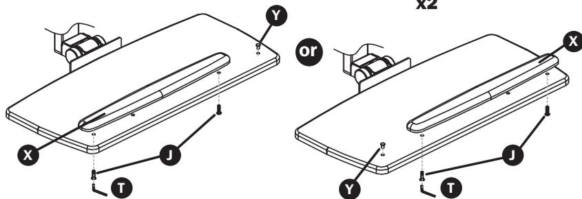
The keyboard Wrist Rest attaches to the left or right side of the Keyboard Shelf to allow for a mouse. If the Wrist Rest is not needed, insert the Plugs to fill the holes.
