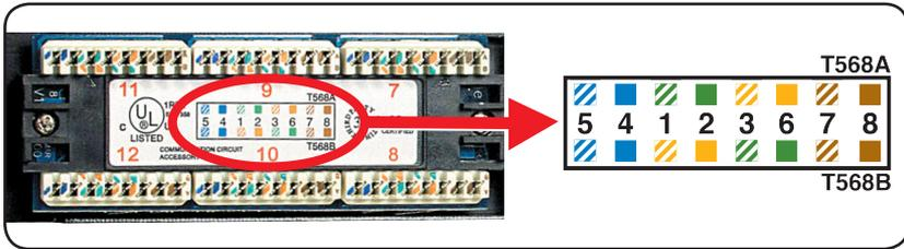
Using the T568A and T568B IDC color codes on the rear panel, connect each respective wire to its corresponding patch panel pin with a punch-down tool.
