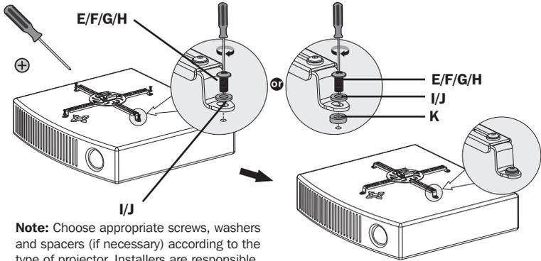
**Note:** Choose appropriate screws, washers and spacers (if necessary) according to the type of projector. Installers are responsible to provide hardware for other types of mounting situations.
