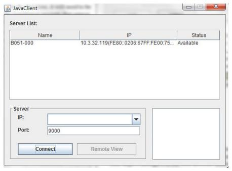
4. If you are on the same network as the B051-000, the client will locate and display it in the *Device List*. In this case, highlight the unit in the device list and click the *Login* button. If you are not on the same network as the unit, it will not be displayed in the list. You must manually enter the IP address in the *IP Address* field, then click the *Connect* button.
