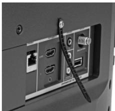
**Note:** If the device does not contain a locking screw, please use the screw included with the cable lock.
