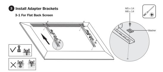
Note: Choose appropriate screws, washers and spacers (if necessary) according to the type of screen.
