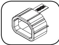
**C14 Plug Sleeve:** (Optional) Use the included C14 plastic sleeves to secure plugs to receptacles. Attach the sleeve to the plug, making sure that the pull tabs remain outside the plug and that the fit is secure. To unplug equipment properly, use the pull tabs to remove the plug and sleeve from the receptacle.
