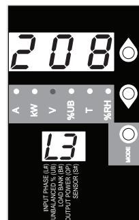
To Unbalanced Load Detect
