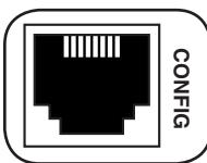
**RJ-45 Configuration Port:** Use this port to provide a direct terminal connection to a computer with a terminal emulation program. An RJ-45 to DB9 cable (part number 73-1243) is included with the PDU. If you need a replacement cable, visit [www.tripplite.com](http://www.tripplite.com) for ordering information.
