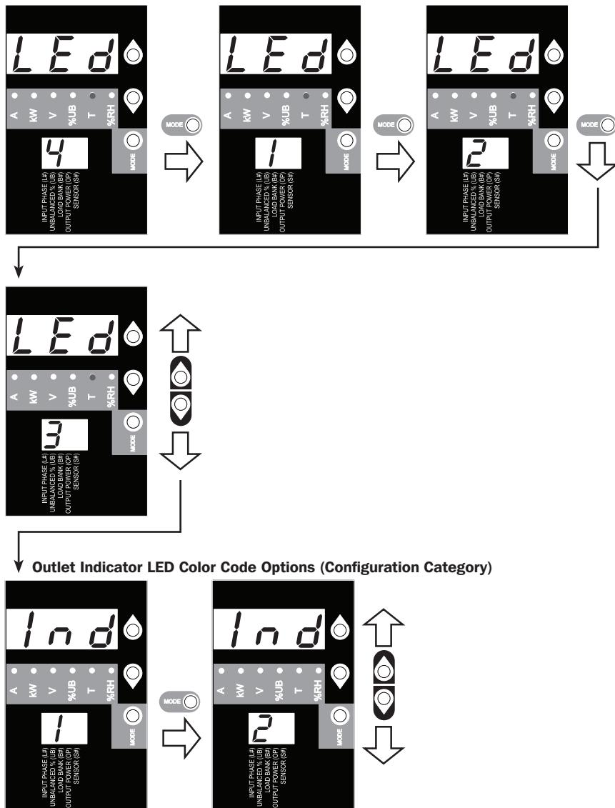
Hold the Mode button for 3 seconds to switch between options.
