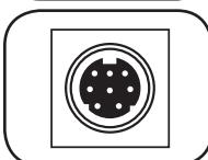
**PS/2 Port:** Use this port to connect a Tripp Lite ENVIROSENSE environmental sensor to provide remote temperature/humidity monitoring and a dry contact interface to control and monitor alarm, security and telecom devices. Visit [www.tripplite.com](http://www.tripplite.com) for ordering information. Note: *Do not connect a keyboard or mouse to this port.*
