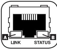
**Ethernet Port:** Use this RJ-45 jack to connect the PDU to the network with a standard Ethernet patch cable. The Link LED **A** and Status LED **B** indicate several operating conditions, as shown in the table below. *This port is not compatible with PoE (Power Over Ethernet) applications.*
