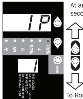
At any point, pressing both of the arrow buttons simultaneously for 1/2 second displays the unit's IP address in the 2-digit display.
