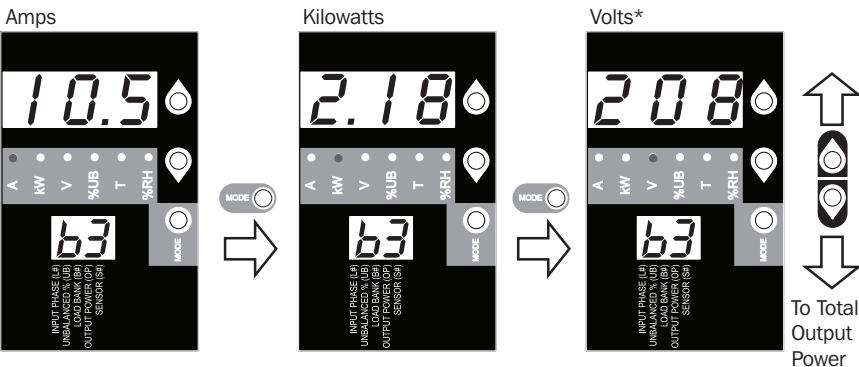
Press Mode button to toggle between options and data within a menu. A momentary press of the arrow buttons switches between menus. A long press skips between measurement categories. The scrolling pattern of the display is outlined below.
