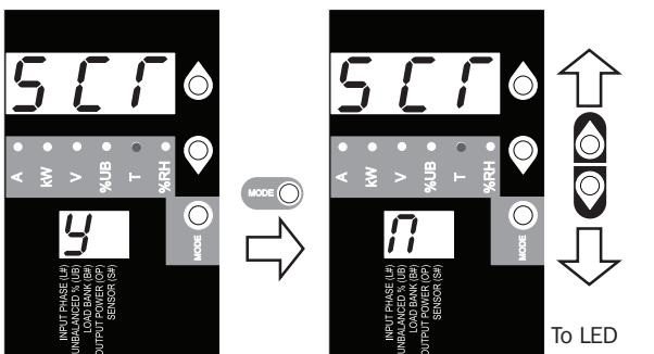
When enabled, the Auto Scroll function displays data for Input Phases, Load Unbalance and Load Banks in 4-second intervals. Y indicates the function is enabled; N indicates that it is disabled. Pressing any button interrupts the Auto Scroll function, allowing the user to navigate between menu options. If no button is pressed, there is a 10 second timeout.
