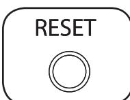
**SNMP Reset Button:** Press the reset button for 3 seconds to reboot the PDU's network card. Rebooting the network card will not erase network settings or interrupt AC power. The reset button is recessed. Use a paper clip or other suitable object to press it.
