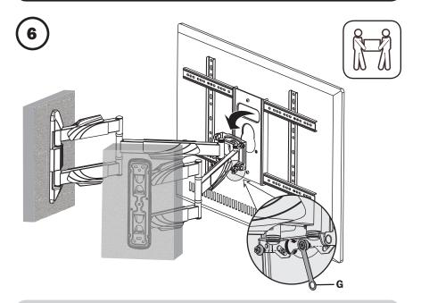
Using an assistant or mechanical lifting equipment, hook the display with attached adapter brackets over the top of the wall-mount bracket. Tighten the bolt on the bottom of the wall-mount bracket to secure the unit.
