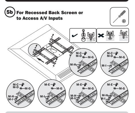
**Note:** Choose appropriate screws, washers and spacers (if necessary) according to the type of screen.
