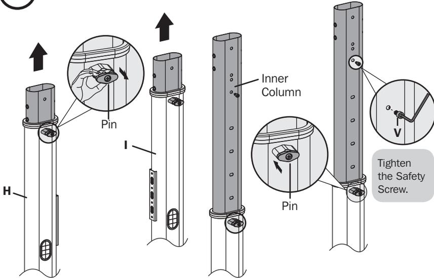
Pull the pin outward and lift the inner column upward at the same time until the inner column is at the desired height. Release the pin to secure.
