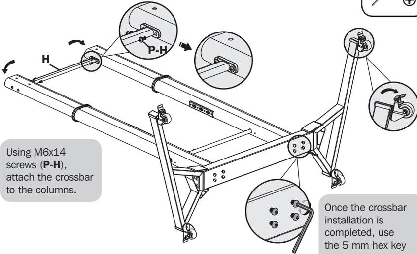
Using M6x14 screws (**P-H**), attach the crossbar to the columns.
