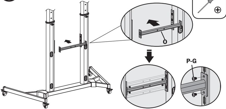
Using M6x8 screws (**P-G**), attach the support bar to the columns at the desired position.
