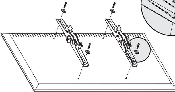
**Note:** Choose appropriate screws and washers according to the type of screen.
