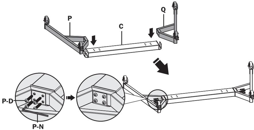
Using M8x40 screws (**P-D**) and the 5 mm hex key (**P-N**), attach the right base to the middle base. Repeat this step for the left base.
