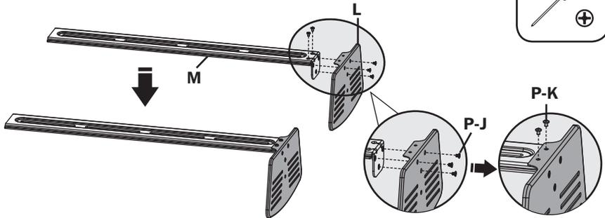
Using M4x6 screws (**P-J**) and (**P-K**), attach the camera shelf to the connecting plate.
