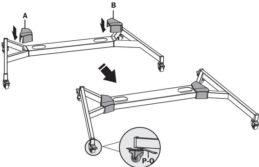
**Note:** Lock the brakes on the casters to avoid any sudden movements during installation. Each caster can be adjusted independently for fine adjustments. Slightly turn each caster nut to lower or raise the base.
