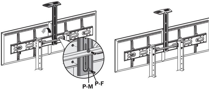
Using M6x25 screws (**P-F**) and D6 washers (**P-M**), attach the connecting plate to the universal plate.
