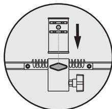
Make sure the bump on **C** and the bolt hole on **B** are matched in alignment.
