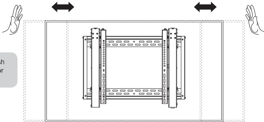
For fast alignment, push the display to the left or right.
