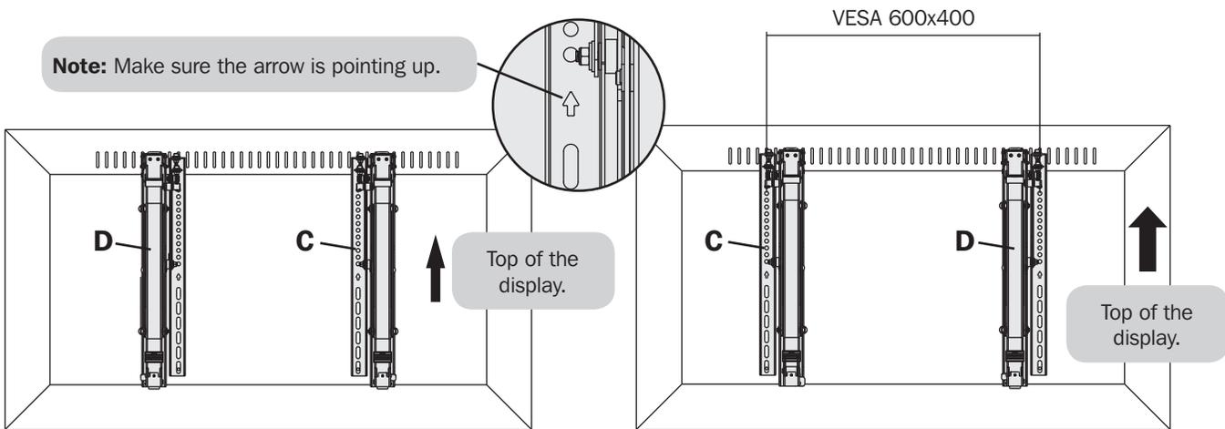
For VESA 600x400 mounting patterns, the "D" and "C" positions are flipped.
