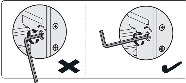
**Note:** Only use the long end of the hex key when tightening the adjustment screws.
