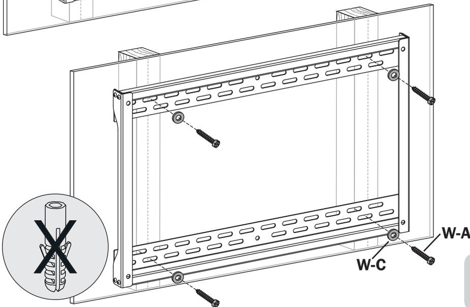
Using the ST6.3x55 screws (**W-A**) and D6 washers (**W-C**), attach wall plate assembly to the wall.
