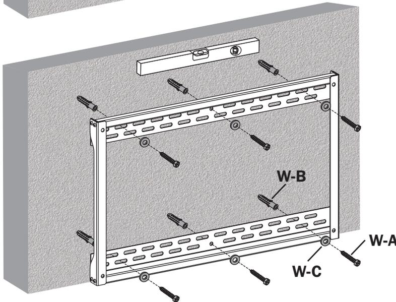
Using the ST6.3x55 screws (W-A), D6 washers (W-C) and concrete anchors (W-B), attach wall plate assembly to the wall.
