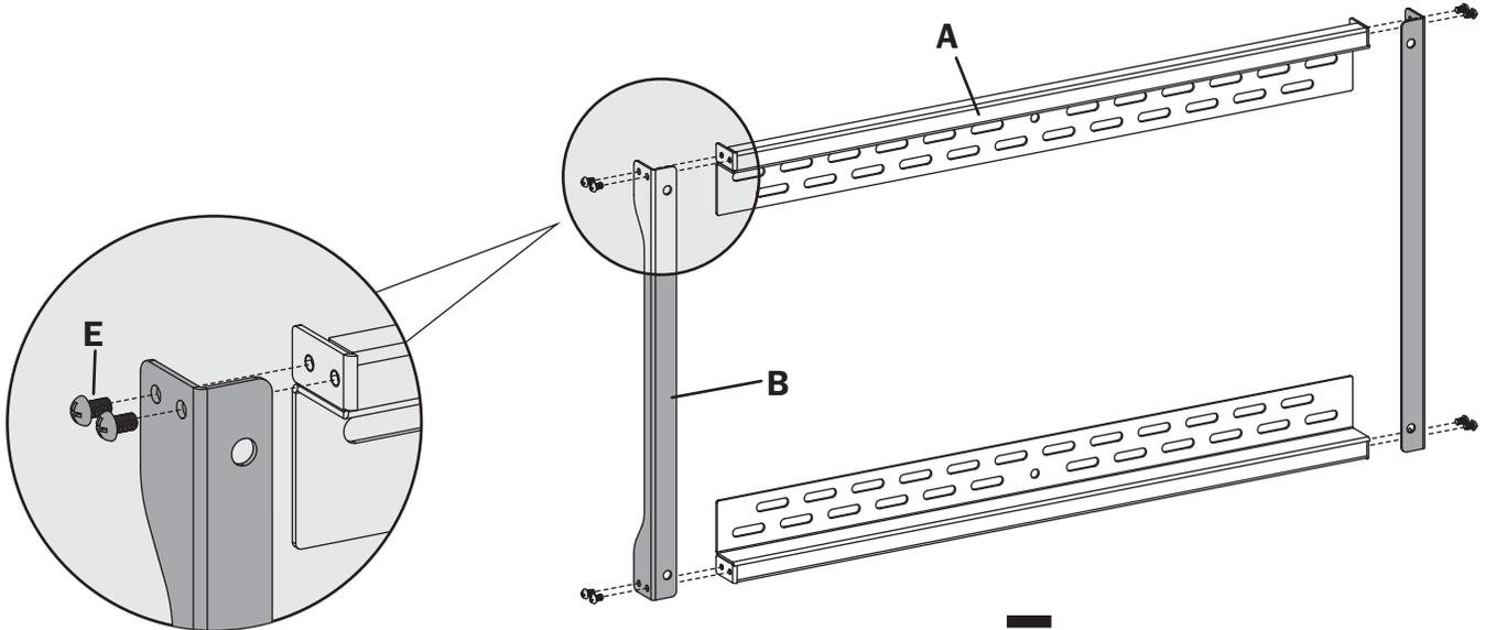
Using the M5x8 screws (E), attach the connecting plates to the wall plates.
