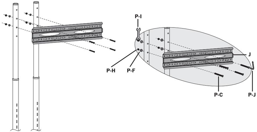
Insert Washers **P-F** and Nuts **P-H** into rear of Telescoping Poles **H** at desired height. Secure Universal Plate **J** with Screws **P-C** using Allen Wrench **P-I**.
