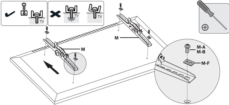
**Note:** Choose the appropriate Screws, Washers and Spacers (if needed) according to the type of screen. Screw the Mounting Arms onto the display.
