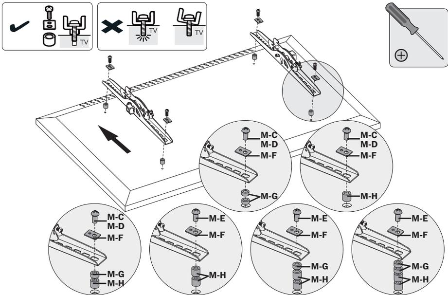
**Note:** Choose the appropriate Screws, Washers and Spacers (if needed) according to the type of screen. Screw the Mounting Arms onto the display.
