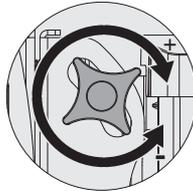
Loosen the knobs to adjust the display to the desired angle.
