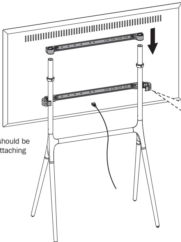
The crossbar should be hidden after attaching the display.
