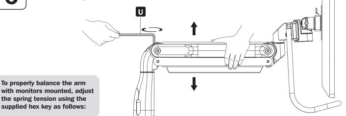
First, position and firmly hold the arm horizontally as shown. Ask for assistance should you require it.
