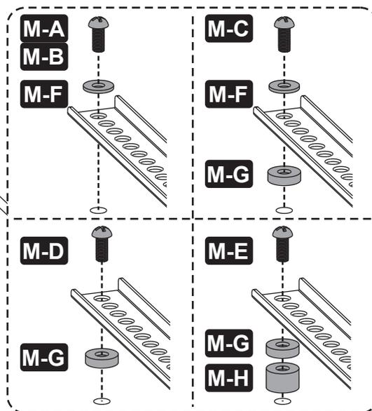
**Note:** Choose appropriate screws, washers and spacers (if necessary) according to the type of screen.
