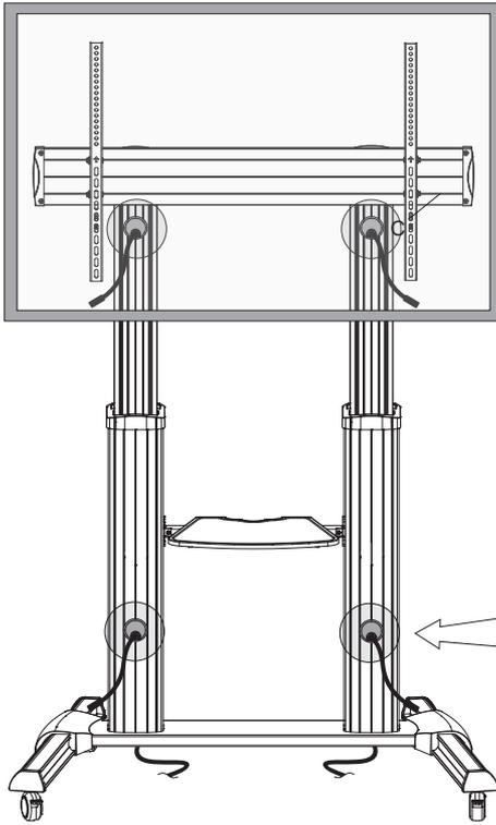
Route the power and connection cables through the openings on the Left and Right Columns.
