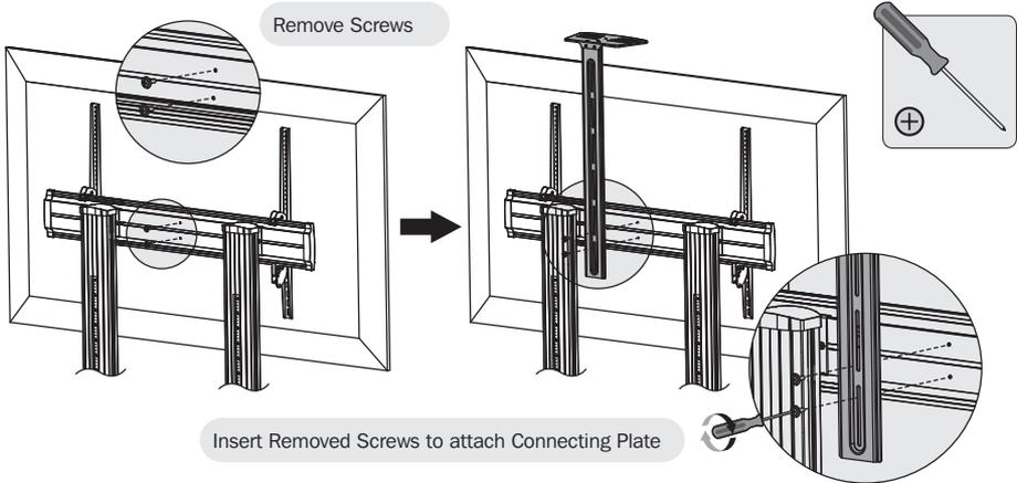
Remove the Universal Plate's two rear screws, then attach the Camera Shelf Assembly using the same screws just removed. Adjust the Camera Shelf Assembly to the desired height, then secure by tightening the screws with a Philips screwdriver.
