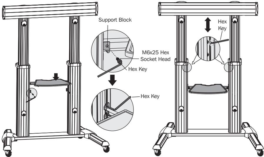
Use the Hex Key and screws to secure the DVD Shelf Assembly to the Columns' Support Blocks.
