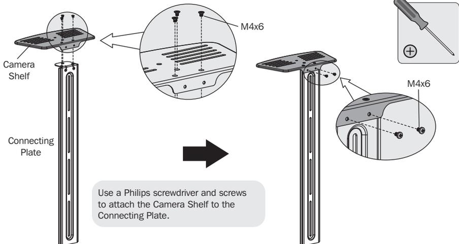
Use a Philips screwdriver and screws to attach the Camera Shelf to the Connecting Plate.
