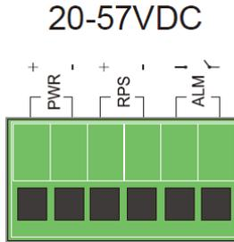
Insert the terminal block connector accessory, which includes “PWR” and “RPS” into the terminal block receptor.
