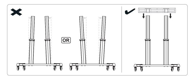
If the columns are not properly aligned, the mouting plate may fail to attach to the columns. Follow the steps below to re-assemble the columns.
