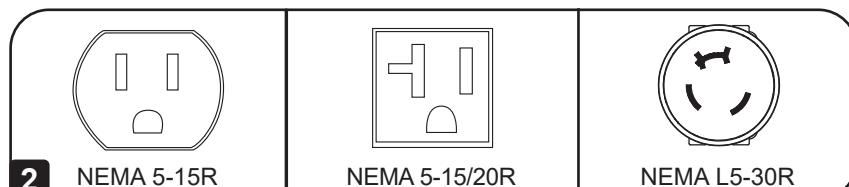
**2** Outlets (Vary by Model): During normal operation, the outlets distribute AC power to connected equipment.
