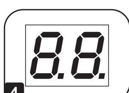
**4** Ammeter (Select Models): The total electrical current used by the PDU will be displayed on the digital meter in amperes (applies only to models equipped with an ammeter).
