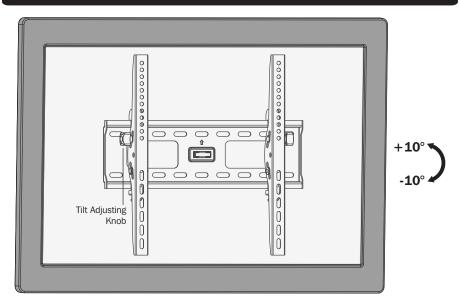
To adjust the tilt angle, loosen the Tilt Adjusting Knobs located on the sides of the adapter brackets. Once the display is at the desired angle, retighten the knobs to hold.
