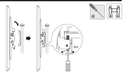
Using an assistant or mechanical lifting equipment, hook the display with attached adapter brackets over the top of the mounted wall plate. Tighten the two screws on the bottom of the adapter brackets to secure the unit.
