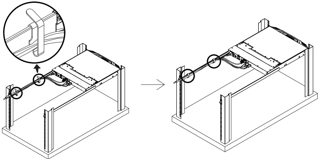
*Note:* It is recommended to manage the cables as tight and space-limiting as possible.
