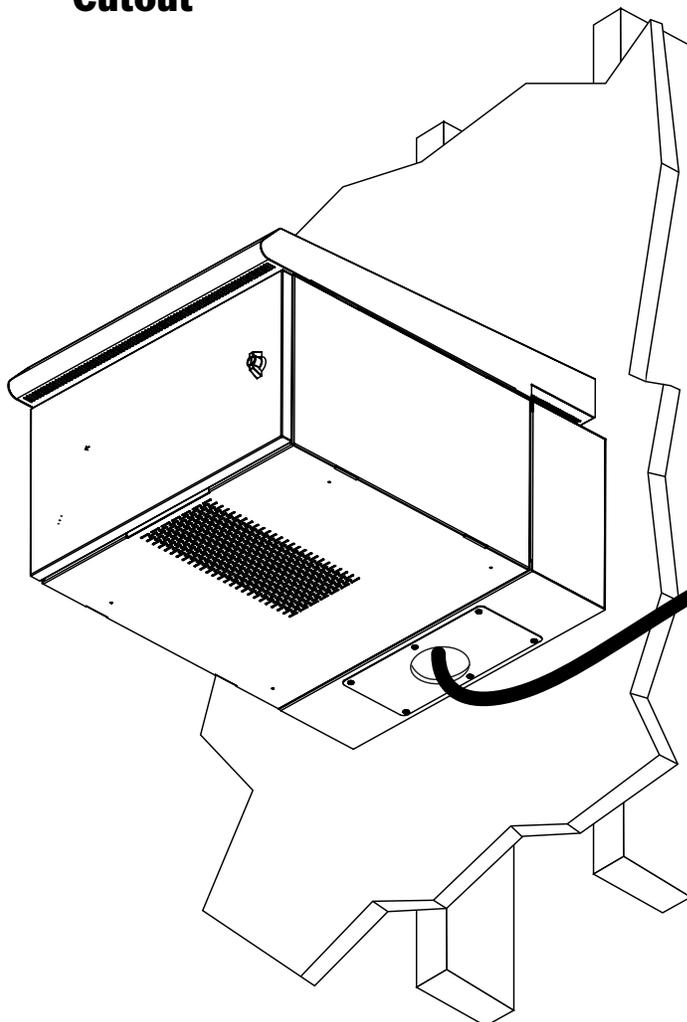
**Note:** To maintain a NEMA rating, use sealed fittings in the cutouts when connecting to conduit. Accessory gland plates with model numbers SRGP1KO, SRGP2KO, SRGP3RM and SRGP4PLASTIC are available (sold separately).
