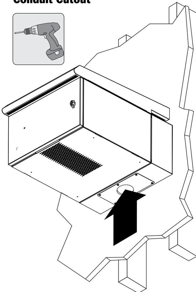
**Note:** This conduit cover supports a maximum Conduit Trade Size 2 with 2.5" hole.
