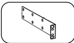
**Longer 1U Mounting Brackets:** Use these brackets to mount the 1U PDU horizontally in a standard rack or rack enclosure. The mounting depth can be adjusted by attaching the brackets to different positions on the PDU.
