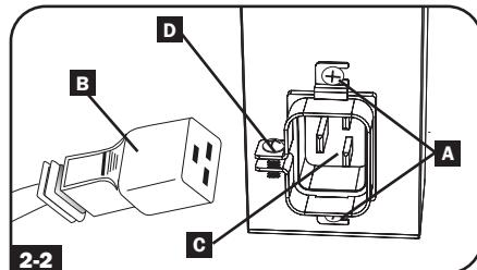
**Note:** When connecting the PDU, it should be provided with over-current protection and a maximum 20A branch-rated over-current protection device.
