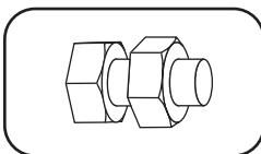
**Grounding Lug:** Use this screw to connect the PDU to ground.
