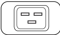
**IEC-320-C19 Output Receptacles:** These two receptacles distribute 208/230V AC power to connected equipment.
