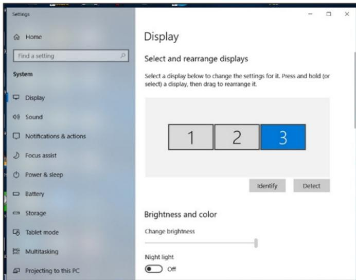
3. Check the Multiple Displays > Extend these displays.
