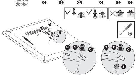
**Note:** Firmly secure the VESA plate to the display using the appropriate screws, washers and spacers (if necessary).
