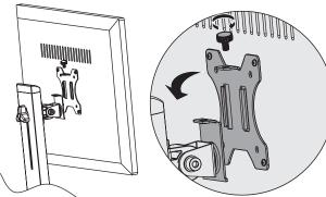
Using an assistant or mechanical lifting equipment, lift the display with attached VESA plate. Slide the VESA plate over the Support Mast bracket. Reattach the top knob to secure the VESA mount (removed in step **1**).
