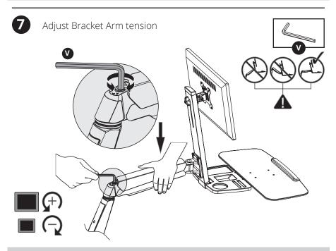
Keep the bracket arm level during tension adjustment. You may need to slightly loosen or tighten the adjustment screw using the provided 6 mm Hex Key, depending on the weight of display installed.
