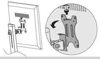
Using an assistant or mechanical lifting equipment, lift the display with attached VESA plate. Slide the VESA plate over the Support Mast bracket. Reattach the top knob to secure the VESA mount (removed in step **3**).
