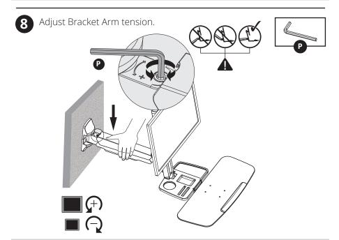
Keep the bracket arm level during tension adjustment. You may need to slightly loosen or tighten the adjustment screw using the provided 6 mm Hex Key, depending on the weight of display installed.
