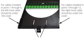
All the cabling should be under the integrated cable loops to prevent the cable from being damaged while being moved in and out.
