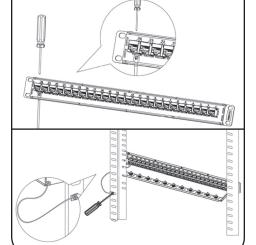
Route the patch cables through the cable manager, securing them with the butterfly clip.
