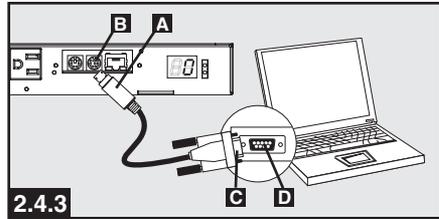
**Connect SNMPWEBCARD to Network:** Connect a standard Ethernet patch cable to the RJ-45 Ethernet port **A** on the card.
