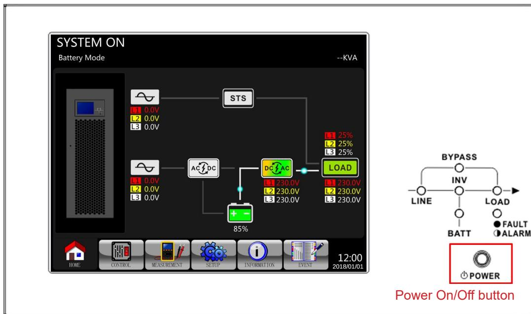
After turning off the UPS, the UPS will transfer to Standby Mode.
