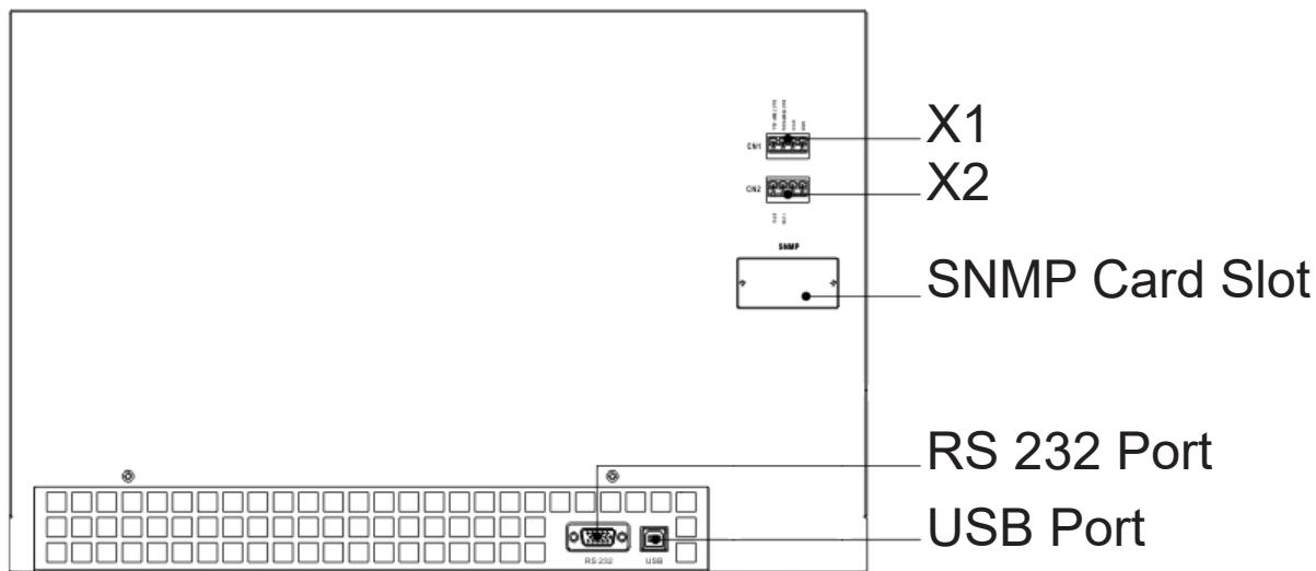
Figure 5.1 Dry Contact Ports and Communication Ports
