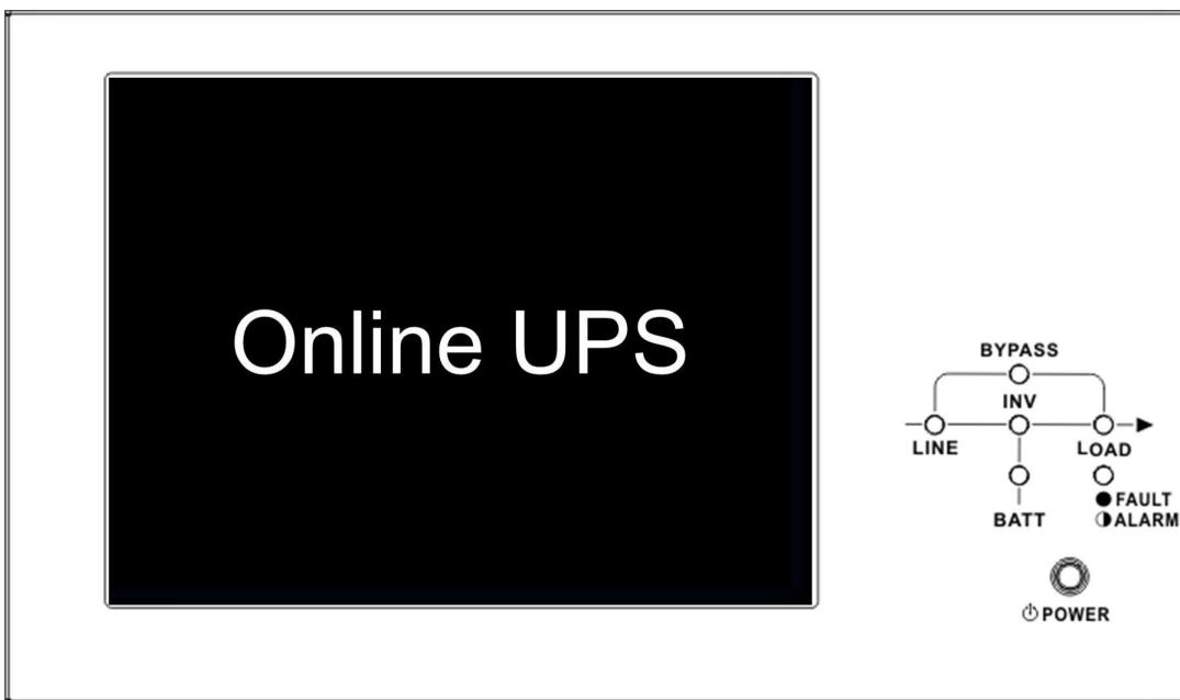
Step 4: While the UPS is displaying the Online screen, immediately press the “Power On/Off” button for 2 seconds until a beep is heard, then release to start the inverter.
