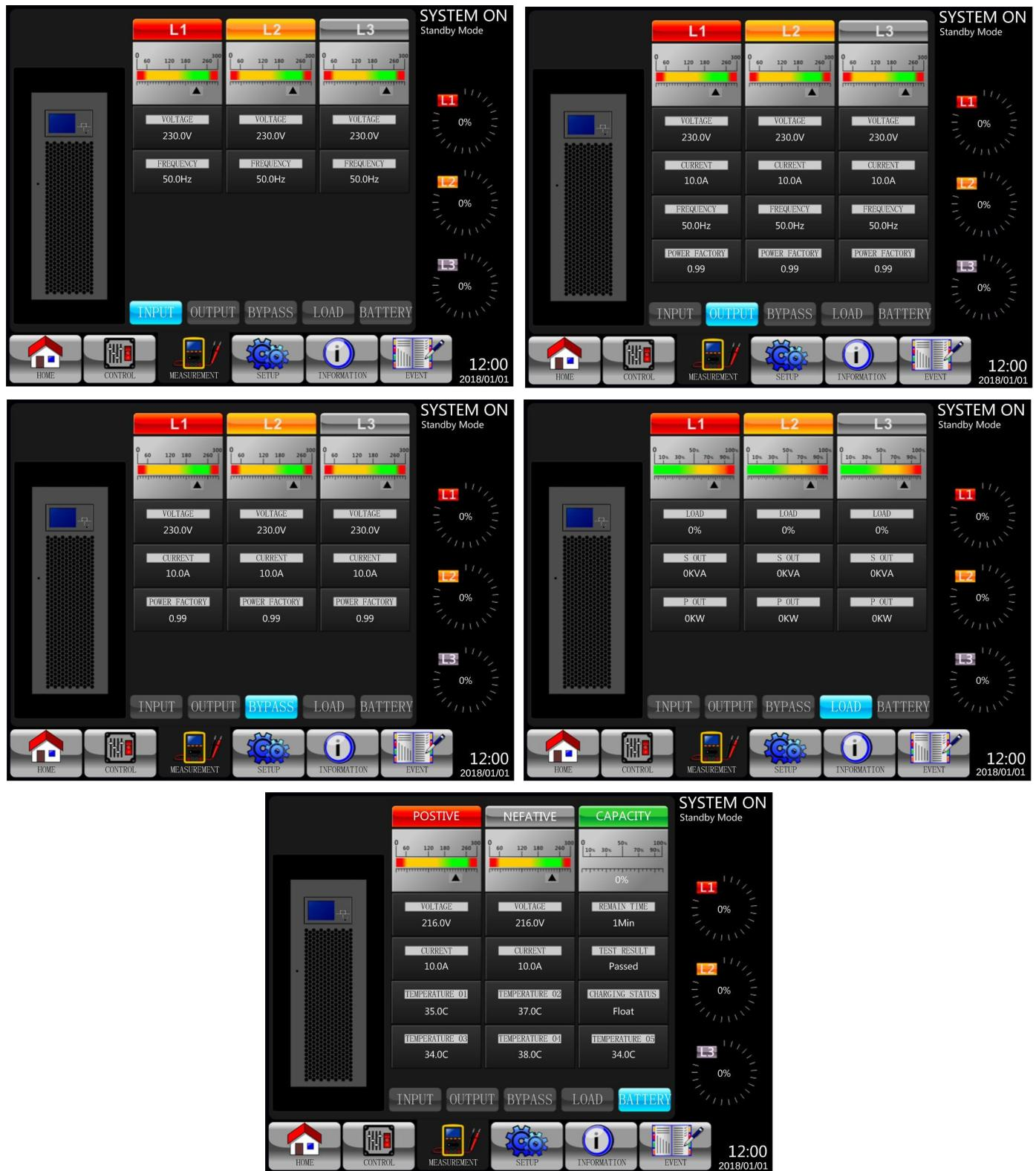
Figure 4.9 Écrans Mesure : INPUT (ENTRÉE), OUTPUT (SORTIE), BYPASS (DÉRIVATION), LOAD (CHARGE) et BATTERY (BATTERIES)
