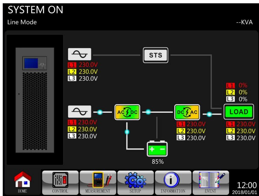
Step 8: The UPS is now in Line Mode. AC startup is now complete.
