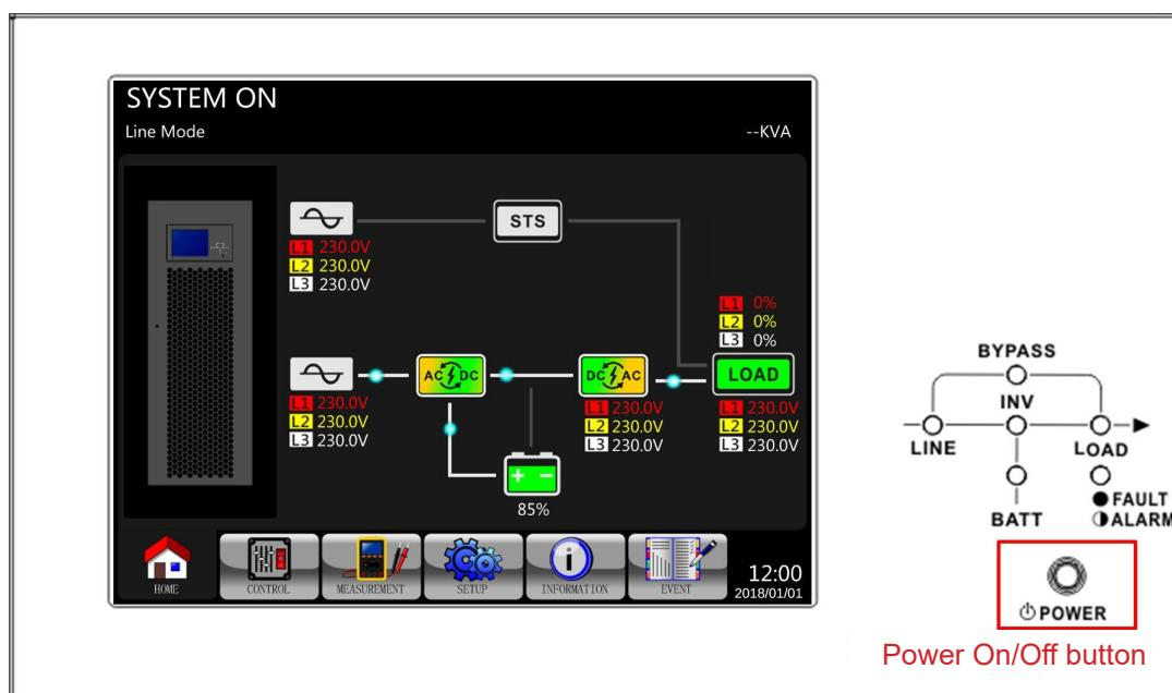
After turning off the UPS, the UPS will transfer to Standby Mode or Bypass Mode, depending on the Bypass Mode setting.
