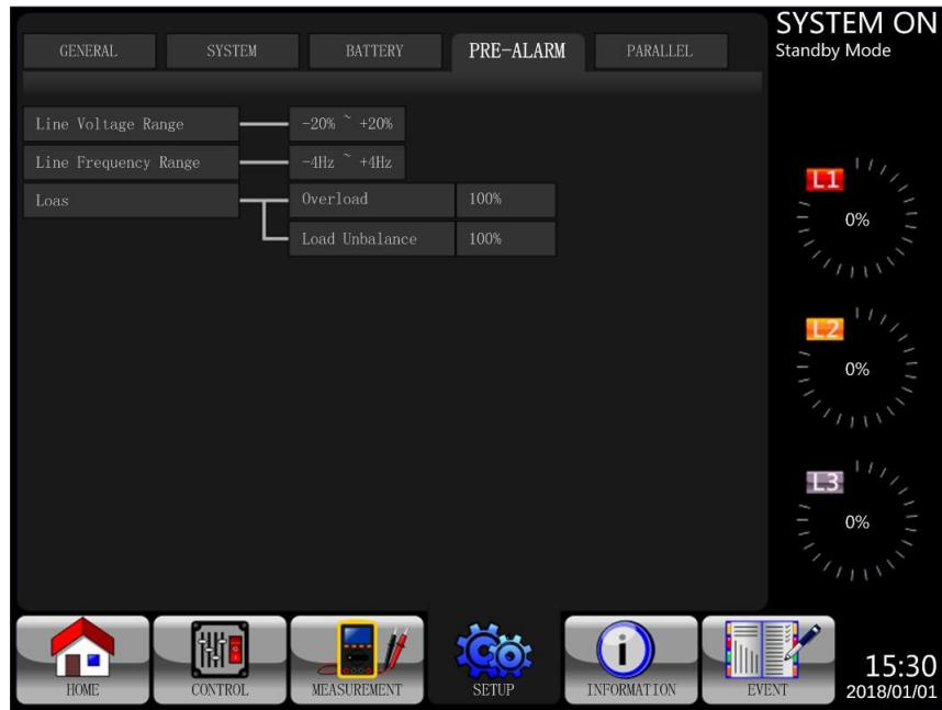
Figure 4.17 Setup-Pre-Alarm Screen
