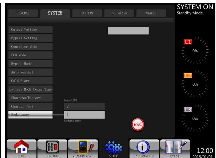
Figure 4.20 Redundancy Across Two Units
