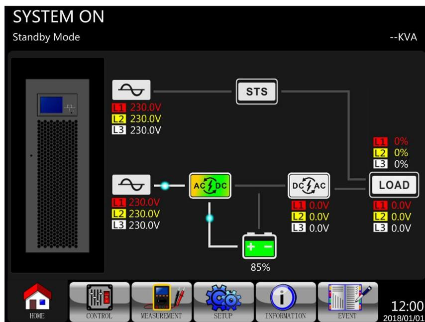
Step 4: Wait one minute. The LCD panel is displayed as shown below. The UPS will enter Bypass Mode if the setting of Bypass Mode is enabled (default setting). If Bypass Mode is disabled, the UPS will remain in Standby Mode.
