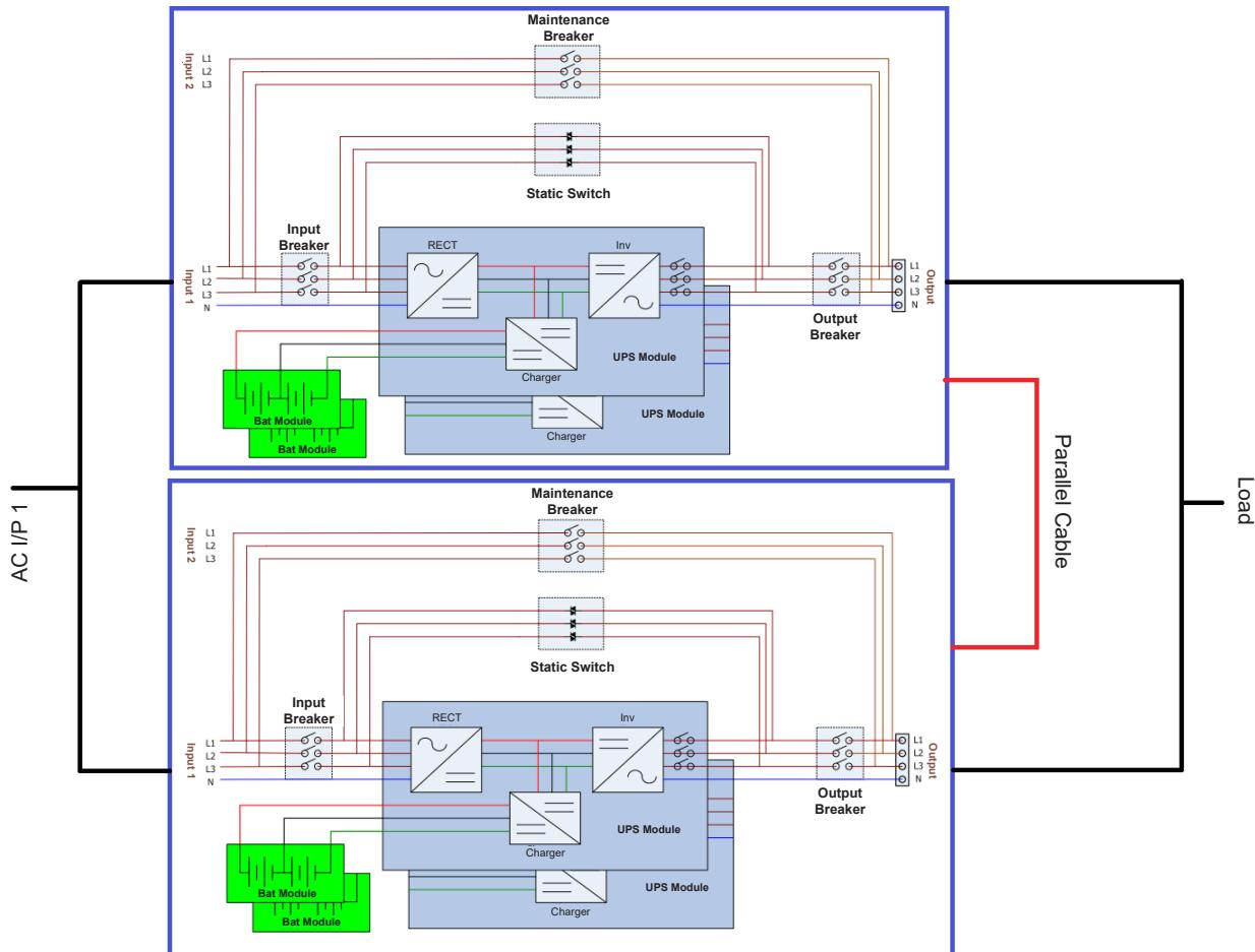
Figure 3.6 Single Input Wiring In Parallel System
