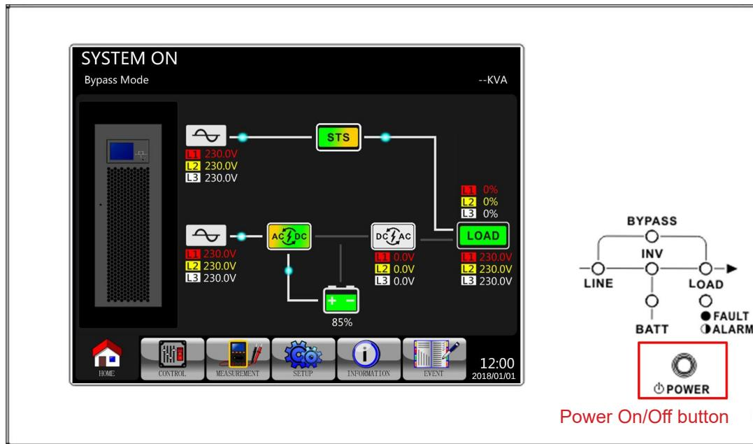
Step 7: Press the Power ON/OFF button for two seconds until a beep is heard, then release to start the inverter.
