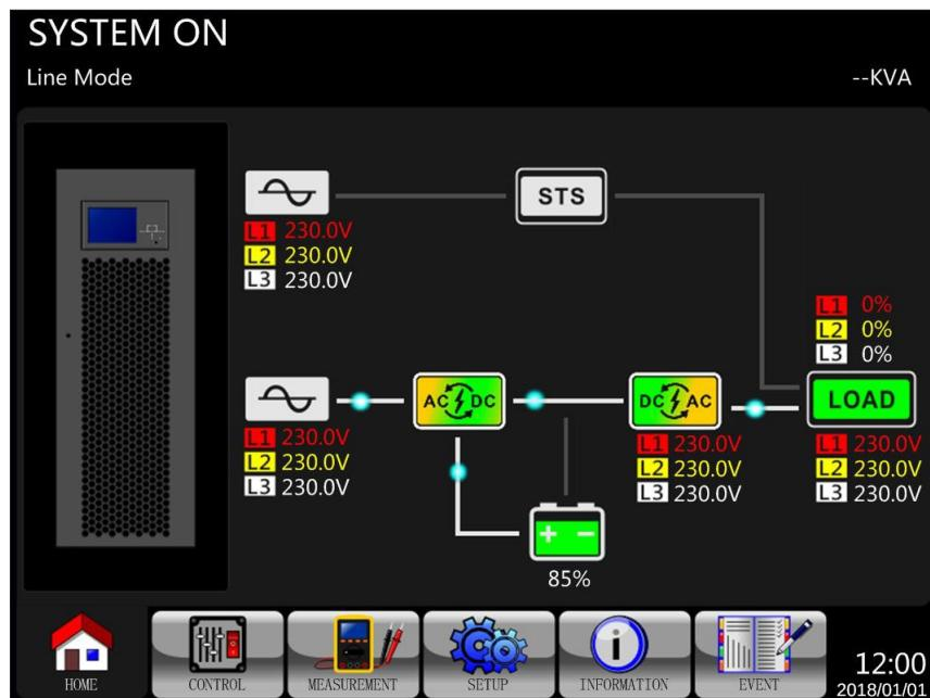
Step 1: Press the “Power On/Off” button for 2 seconds until a beep is heard to turn off the UPS, or use the Menu-Control-System Turn Off to turn off the UPS.
