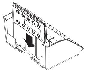
**B** Connect the AC power cables appropriate for the number and type of devices. The slots located at the top and front of the enclosure base allow for convenient cable routing.
