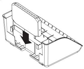
C Connect USB charging cables appropriate for the number and type of devices. The slots located at the top and front of the enclosure base allow for convenient cable routing.
