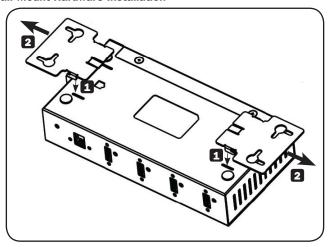
To install the wall-mount brackets, insert the bracket tabs into the slots on the bottom of the unit 1 and then pull outward to lock into place 2.
