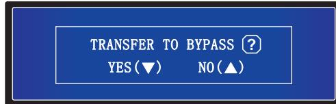
In battery mode, press the OFF key ( **OFF** ) once. To turn off the UPS, press the DOWN key (
