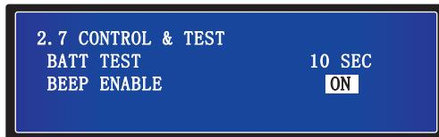
1. **BATT TEST:** Enable or disable battery test. Three are three choices: **ABORT**, **DEEP** or **10 SEC**.
