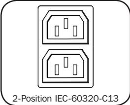
**Outlets (Vary by Model):** During normal operation, the outlets distribute AC power to connected equipment. Select models feature an LED that indicates outlet status.
