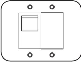
**Circuit Breakers (Select Models):** If the connected equipment load on a load bank exceeds the Maximum Load Rating of the load bank, the circuit breaker will trip. Disconnect excess equipment and switch breaker to the on position to reset the breaker. Models with multiple outlet banks have a circuit breaker for each bank. Circuit breakers are only used to protect output load banks.
