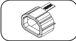
**C14 Plug-Lock Inserts (Optional):** Use the included C14 plug-lock inserts to secure plugs to C13 receptacles. Attach the sleeve to the plug making sure the pull tabs remain outside the plug and that the fit is secure. To unplug equipment properly, use the pull tabs to remove the plug and insert from the receptacle.
