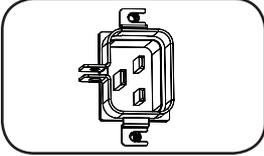
**Power Inlet (Select Models):** The IEC power inlet connects to the included power cord or a compatible user-supplied power cord. The inlet includes a bracket to secure the cord connection.
