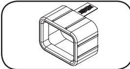
**C20 Plug-Lock Inserts (Optional):** Use the included C20 plug-lock inserts to secure plugs to C19 receptacles. Attach the sleeve to the plug making sure the pull tabs remain outside the plug and that the fit is secure. To unplug equipment properly, use the pull tabs to remove the plug and insert from the receptacle.
