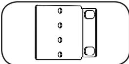
**Mounting Brackets:** Use these brackets to mount the PDU.
