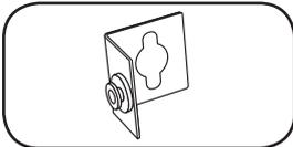
**PDUMVROTATEBRKT Mounting Accessory:** Use these V-shaped brackets to mount the PDU with its outlets facing the rear of the rack.
