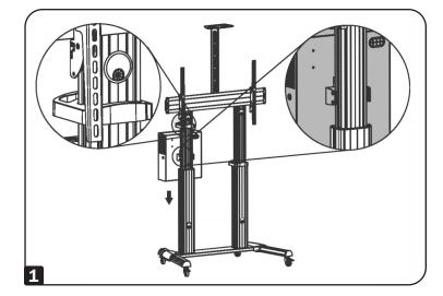
2 Slide the enclosure down the column by inserting the bracket's screws into the channels on each side of the column.
