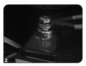
3 Secure the yellow ground lug and the black negative (-) battery lug to the black negative (-) battery terminal using the stud. Slide the black terminal cover over the terminal post.
