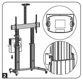
**3** Adjust the height of the enclosure and firmly tighten the screws on each side of the bracket.
