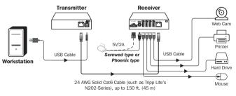
**Note:** When connecting the receiver to power-hungry device(s), add external power (5V 2A) via its Phoenix connector.
