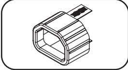
**C14 Plug-Lock Insert Sleeve (Optional):** Use the included plastic sleeves to secure C13 power cords to C14 inlets. Fit the sleeve over the end of the cord, making sure the pull-tabs remain outside the cord and the fit is secure. To unplug equipment properly, grip both the cord and the insert's tabs at the same time and pull.
