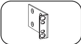
**Mounting Brackets:** These detachable brackets enable the PDU to be installed in a 2U rackmount configuration or an under-counter configuration.
