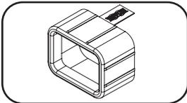
**C20 Plug-Lock Insert Sleeve (Optional):** Use the included plastic sleeves to secure C19 power cords to C20 inlets. Fit the sleeve over the end of the cord, making sure the pull-tabs remain outside the cord and the fit is secure. To unplug equipment properly, grip both the cord and the insert's tabs at the same time and pull.
