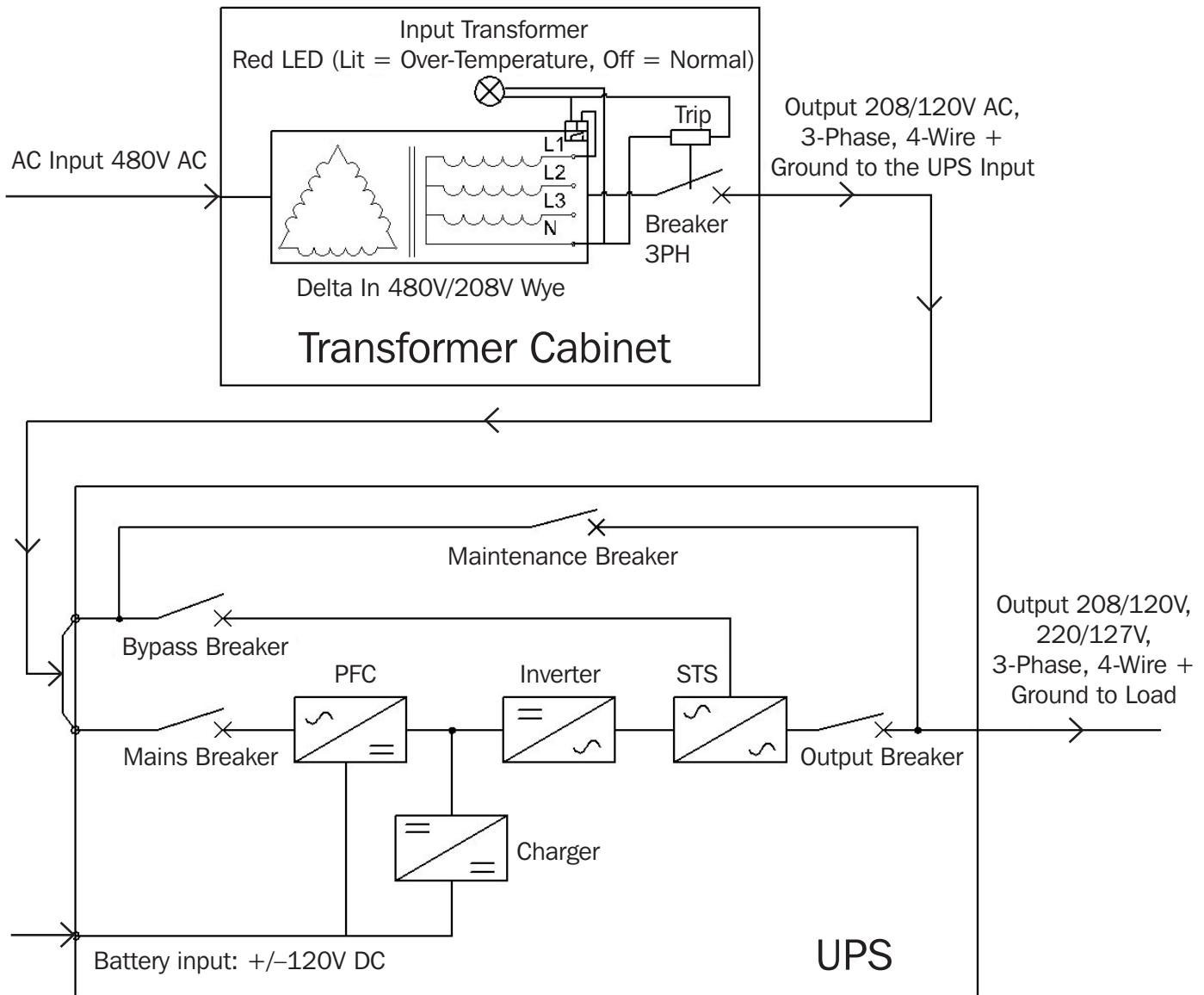
Figure 3-7: Connection Line Diagram for S3MT-60K480V / S3MT-100K480V
