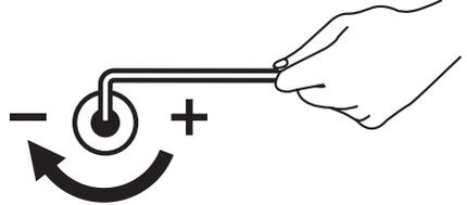
If the arm **rises**, turn the adjustment screw **clockwise** until it stays in a horizontal position.
