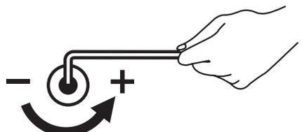
If the arm **drops**, turn the adjustment screw **counter-clockwise** until it stays in a horizontal position.
