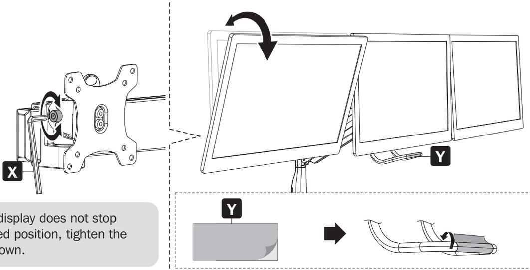
**Note:** If the display does not stop at your desired position, tighten the screws as shown.
