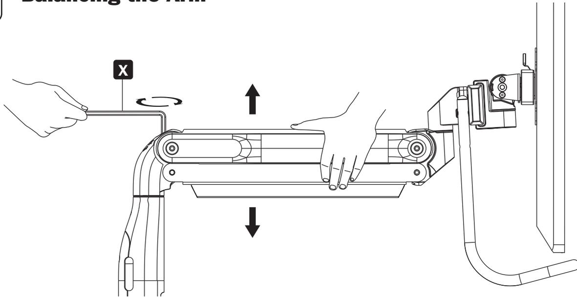
To properly balance the arm with monitors mounted, adjust the spring tension using the supplied hex key as follows:
