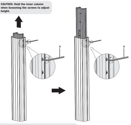
Adjust inner Column J to the desired height, then tighten all screws.
