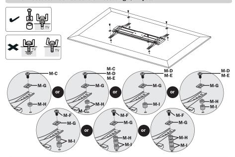
**Note:** Choose the appropriate Screws, Washers and Spacers (if needed) according to the type of screen. Screw the Adapter Brackets onto the display.
