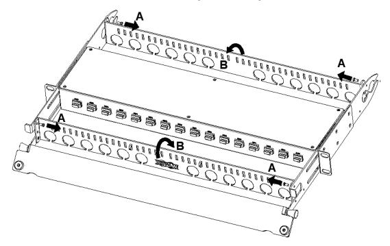
Step 3: Mount the panel into an EIA-standard 19-inch rack, and secure the screws.
