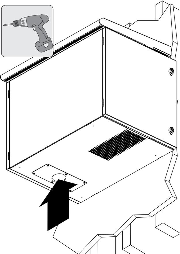
**Note:** This conduit cover supports a maximum Conduit Trade Size 2 with 2.5" hole.
