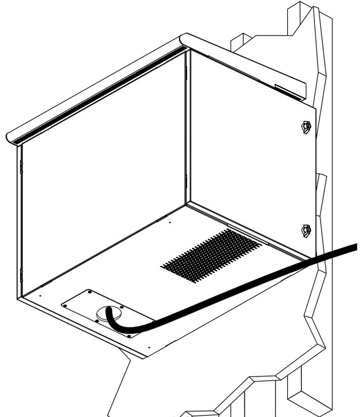
**Note:** To maintain a NEMA rating, use sealed fittings in the cutouts when connecting to conduit. Accessory gland plates with model numbers SRGP1KO, SRGP2KO, SRGP3RM and SRGP4PLASTIC are available (sold separately).
