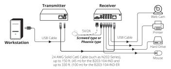
**For the B203-101/104-IND models only:** when connecting power-hungry device(s), use either the included external power supply or RS-232 Phoenix connector to add external power.
