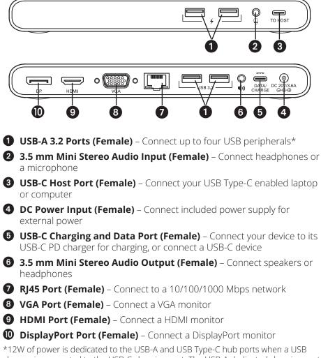
charger is connected to the USB-C charging port. The USB-A dedicated charging port supports 5V 1.5A (7.5W). When maxing out one port's power, the other ports' power is reduced. All ports will not be able to provide full power simultaneously, meaning external power may be required for some connected peripherals.
